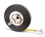
The closed reel steel long tape features a rugged rewind mechanism. Nylon rollers at case opening to reduce blade wear through sustained field use. Blades are produced with high visibility, easy-to-read graduations.
